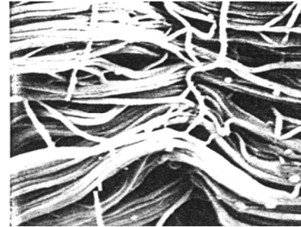
EM image highlighting the importance of the specimen orientation before performing a biomechanical test
